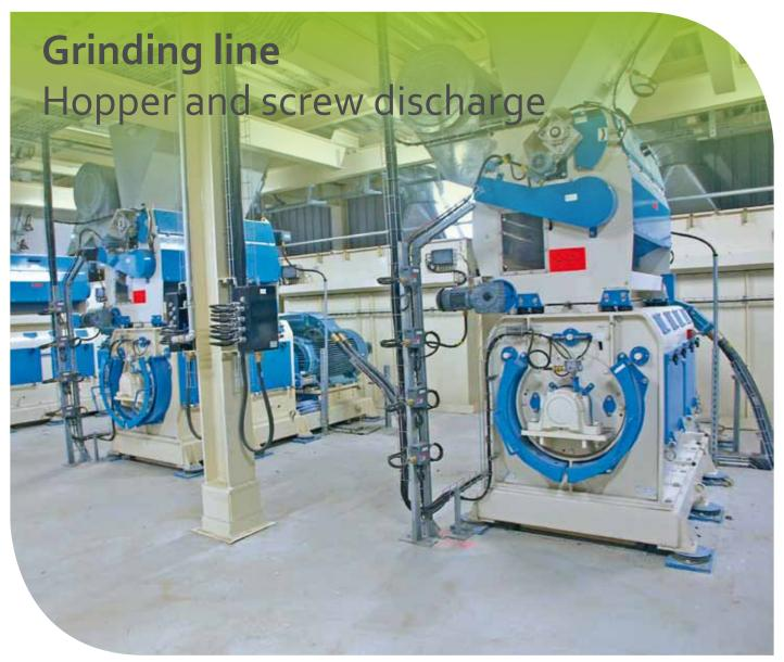
The RMP or RMA type hammermills are generally installed on a concrete or metal floor and fixed with anti-vibrating mountings.
