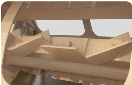
Rotor with pre-adjusted paddles
